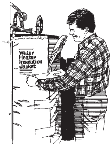
A water heater blanket on an older heater can save up to 9% of your water-heating costs.
